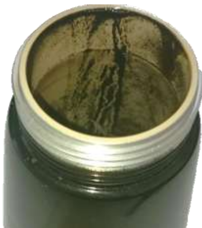
Example of residue built up in cream charger used to dispense N2O | FEB 16
